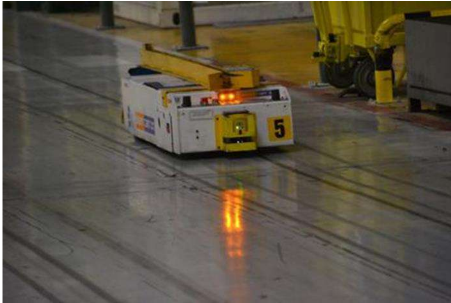
Figure 3: Design of AGV for internal transport in logistics
