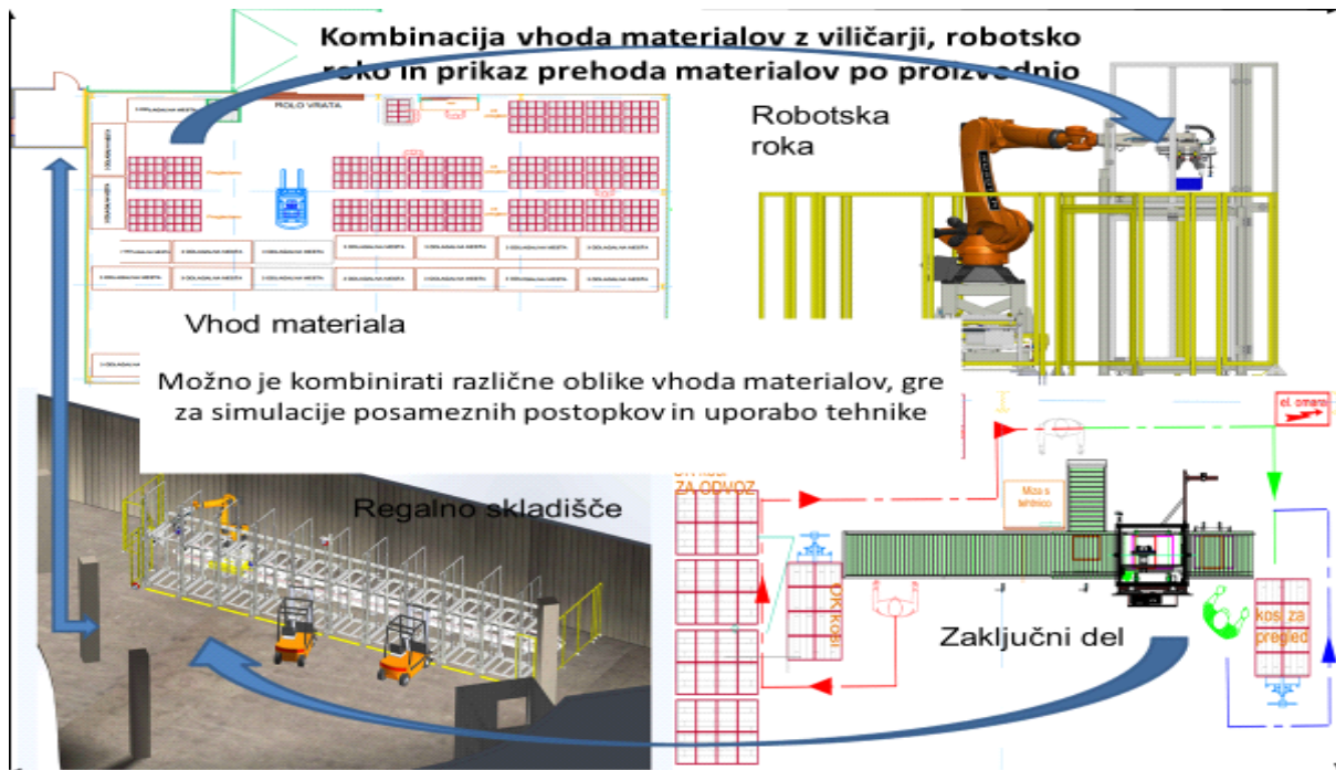
Picture 2: Combination system of receiving material and their way through production
